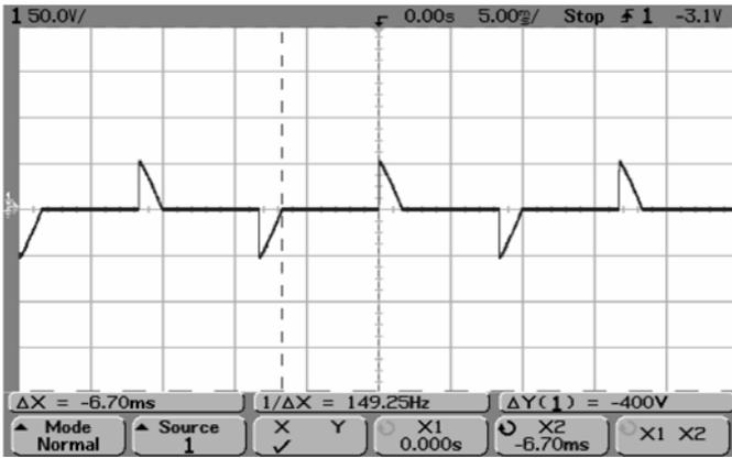
Figure 6: Firing angle = 145°
