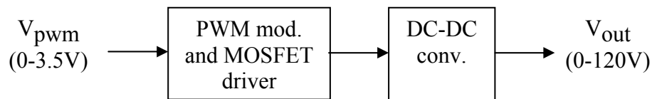
Figure 1. Block Diagram of the Open Loop DC-DC Converter “Process”
