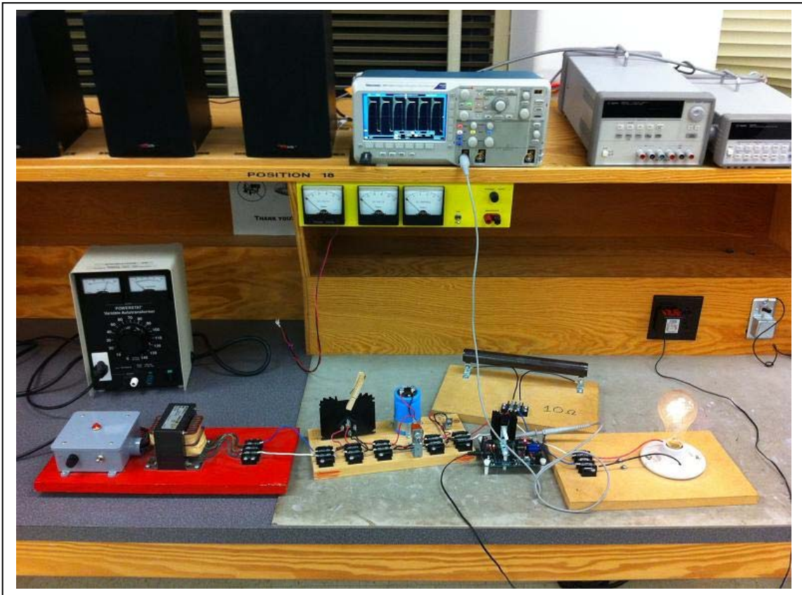
Figure 12: Full Set-up of MOSFET testing depicting Variac, 115:25 Iso Transformer, DBR, 10\ \Omega load & light bulb load in parallel, and MOSFET switch on low-voltage side of dc bus
