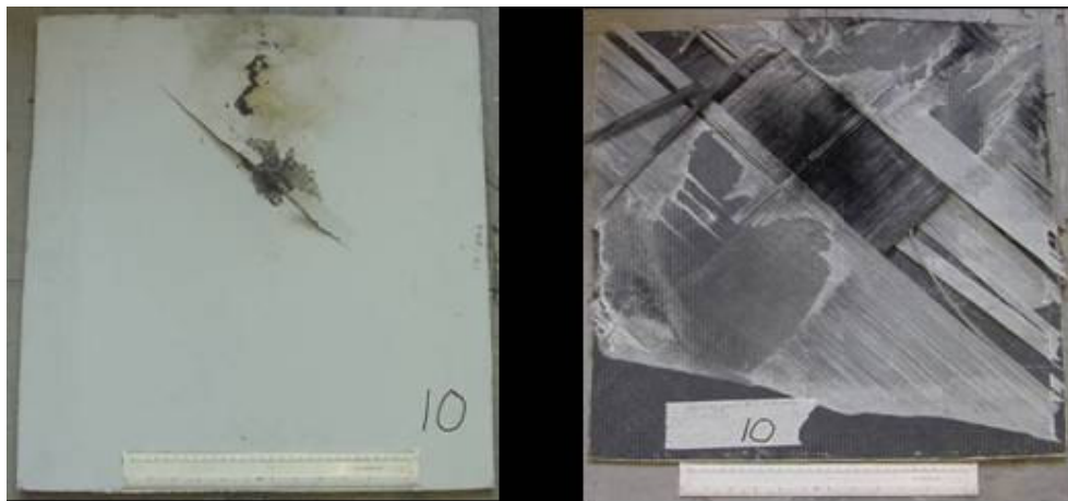
Figure 13.3: Blade Mid-section (without I/s protection) after High Current Testing
