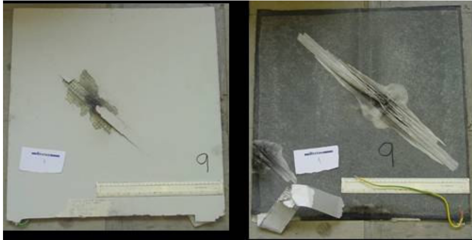
Figure 13.2: Blade Mid-section (with I/s protection) after High Current Testing
