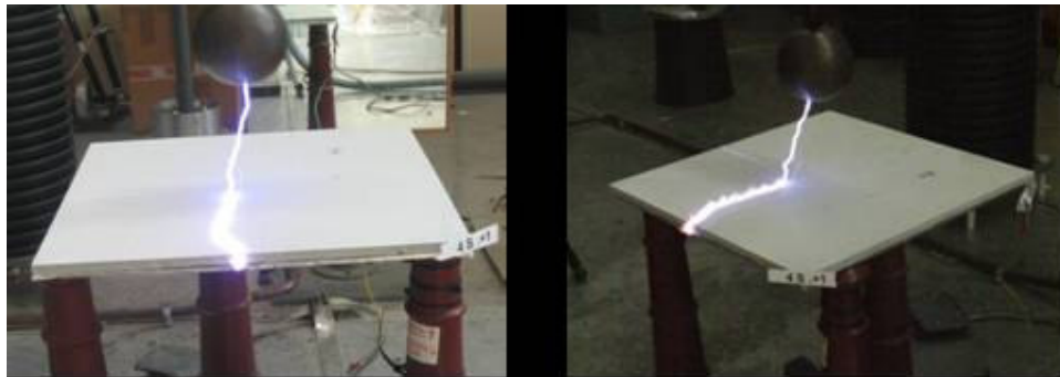
Figure 13.1: Blade Leading Edge Test Panel during High Voltage Testing
