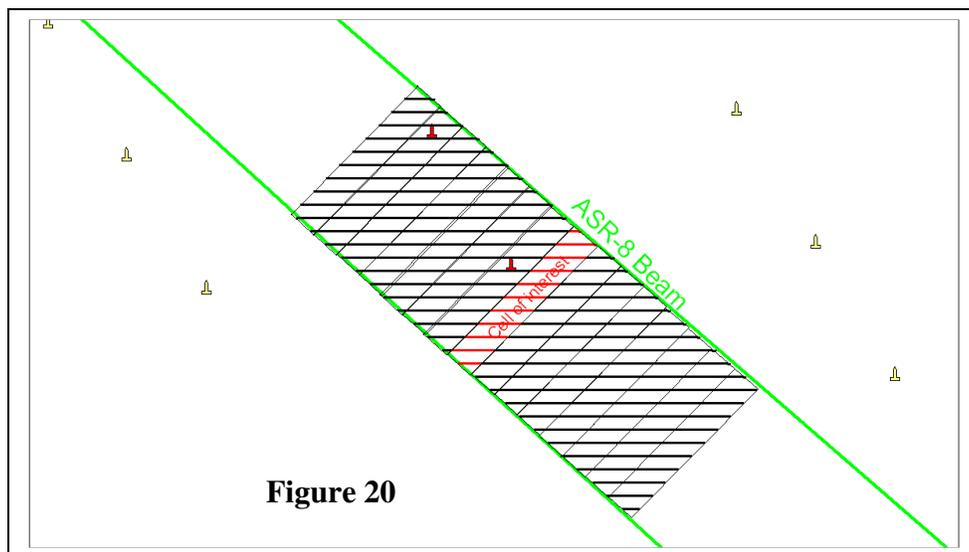
7\* 1/16nm wide range cells on either side of the cell of interest are used in the CFAR calculation. The radar will typically see groups of 2 or 3 wind turbines .3nm apart with 1nm between each group. This will result in the threshold being raised over most of the wind farm when the wind is blowing in a direction that would result in clutter.
