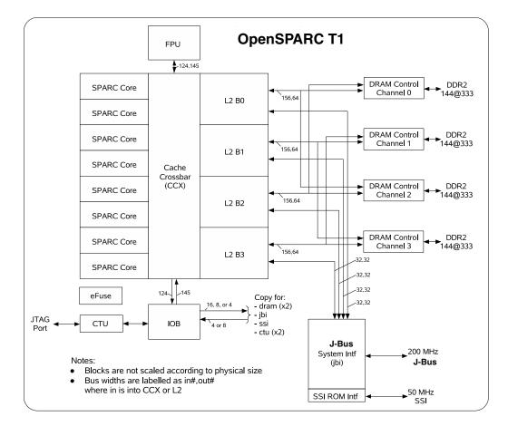
FIGURE 1-1 OpenSPARC T1 Processor Block Diagram
