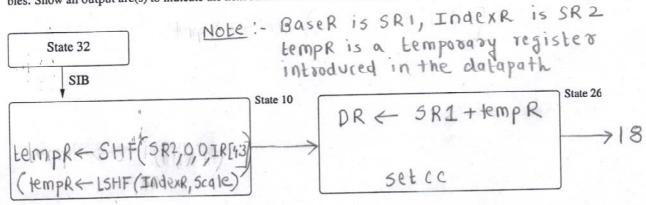
Using the data path diagram labeled "SIB with two extra states" on the next page, add any additional structures and any control signals needed to implement SIB as specified by the two states shown in the bubbles. Label any additional control signals "ECS 1" (for "extra control signal 1"), "ECS 2" etc.
