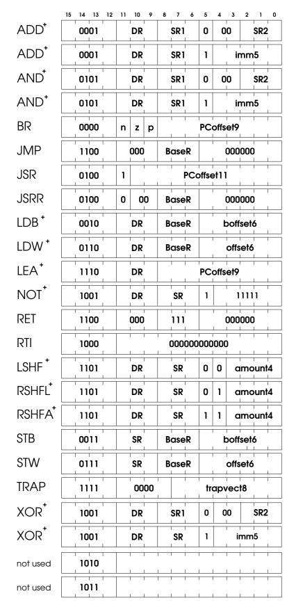
Figure 1: LC-3b Instruction Encodings
