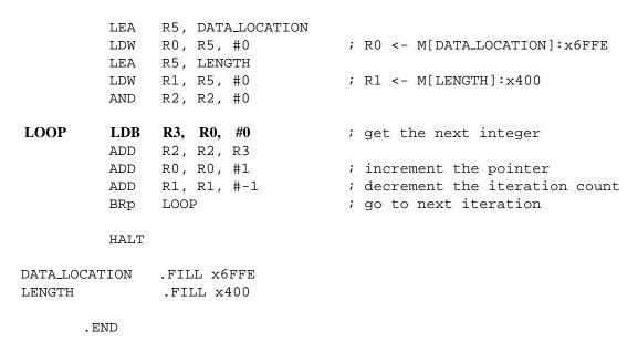
Assume the program executes on an implementation of the LC-3b that supports virtual memory. The 16-bit addresses you are familiar with are virtual addresses. Physical memory is 8KB. Page size is 512 bytes.
