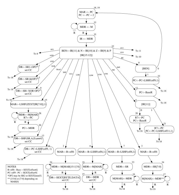
Figure 2: A state machine for the LC-3b
