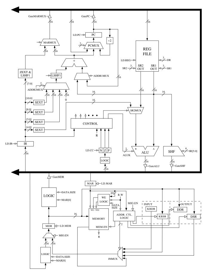
Figure 3: The LC-3b data path
