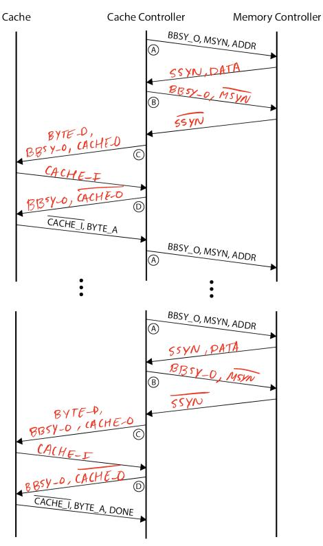
**Part b** (10 points): Complete the state machine for the cache controller by filling in the bolded boxes showing how it loads a cache line from memory in one bus cycle.
