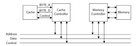
Your job is to implement the state machine for a cache controller so it can load a cache line from memory in one bus cycle. A cache line consists of eight bytes.
