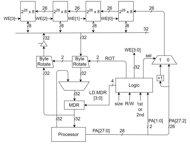
Both byte rotators in the figure are right rotators.
