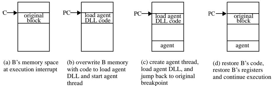
Fig. 3. "Code Patching" an Agent into Binary B
