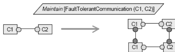
Figure 3.2: Fault-tolerant refinement pattern
