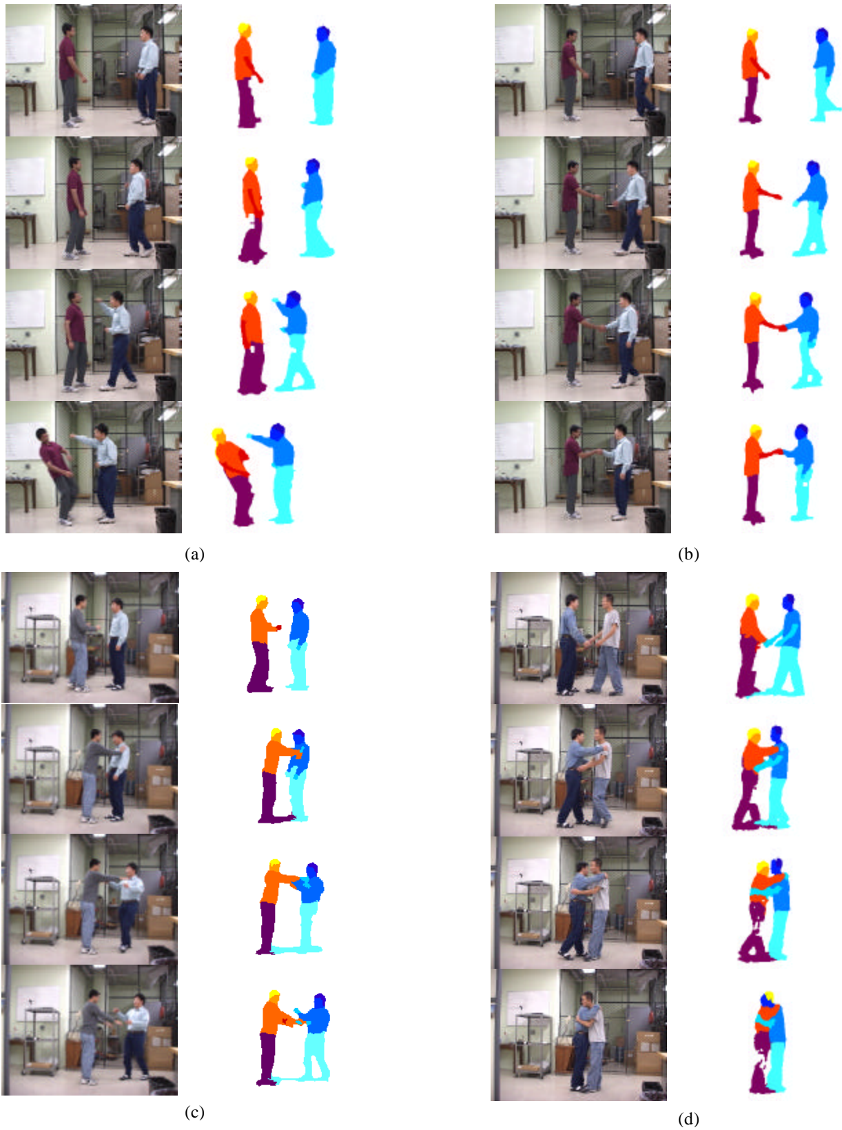
Fig. 6. Example input sequences (1 st column) and the corresponding sequences of tracked body parts (2 nd column). (a) 'punching', (b) 'hand-shaking', (c) 'pushing', (d) 'hugging'. Degree of occlusion increases from (a) to (d). The consistency of grayscale (which is color in the original version) of the individual blobs in the 2 nd columns in each sequence indicates that each person is correctly tracked and that the interacting persons' individual body parts are correctly segmented and tracked despite of occlusion, shadow, and foreground pixel loss.
