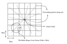
Fig. 1. Forwarding packets along straight lines - We require only one transmission per tile for broadcasting.
