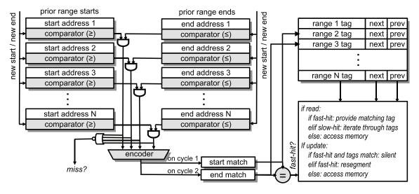
Figure 2: Range Cache Architecture: The first pipeline stage matches the start and end points of the new range, while the second stage is a state machine that performs tag lookup and decides on the aggregated range entry to be written back.
