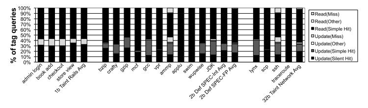
Figure 5: The relative proportion of various range queries for Dataflow Tracking. The SPEC applications (bzip through wupwise) are run with the definedness tracking tool, while the Ruby applications (admin login through store view) and network applications (lynx through traceroute) are run with network input taint tracking. The vast majority of accesses fall into "fast" categories where the updates are simple and the reads are hits to a single range.
