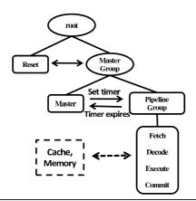
**Figure 8.** State Machine Diagram of the Coarse-Grained Time-multiplexed Pipeline. The memory hierarchy shown in the dash box does not represent any concrete state in the state machine, but it is included in our CPU and accessed by the pipeline.
