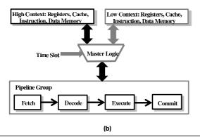
**Figure 9.** Synthesized hardware implementation of the Coarse-Grained Time-multiplexed Pipeline CPU logic when the entire pipeline is multiplexed between *high* and *low* code.
