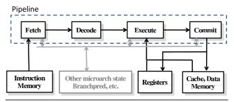
**Figure 7.** A typical CPU pipeline and its interaction with memories, registers and other components. Our CPU design implements all parts in **bold**.
