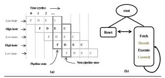
**Figure 12.** Fine-Grained Pipeline Multiplexing. (a) Intuition behind the design (b) State Machine Diagram
