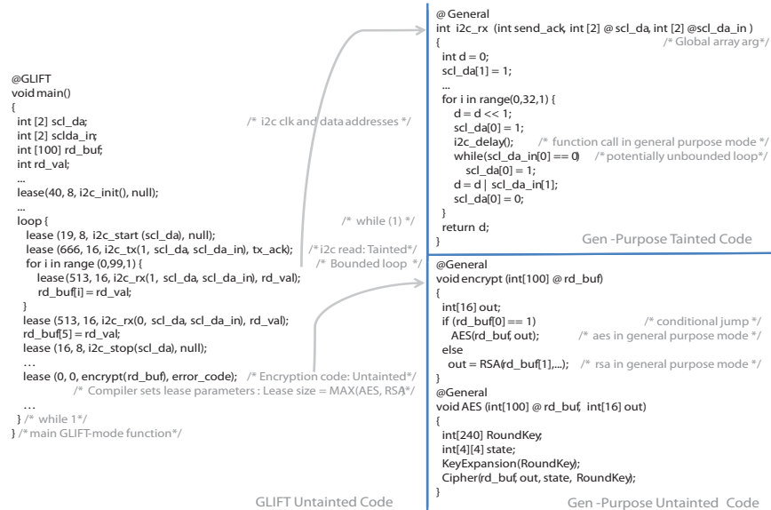
Figure 10: Programming using Execution Leases: Execution begins in trusted (untainted) GLIFT mode. Function calls can be made to general-purpose functions that operate within a fixed time and memory lease. Within a lease, general purpose code can execute conditionals (without predication), potentially unbounded loops, and communicate through protected memory regions, while the CPU implementation guarantees that no tainted code can ever interfere with out of bounds memory or execution time.
