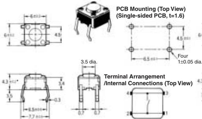
\* The height of B3F-1020, B3F-1022, B3F-1025, and B3F-1026 is  $5 \pm 0.2$  mm.
