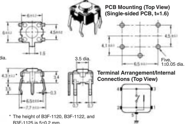
\* The height of B3F-1120, B3F-1122, and B3F-1125 is  $5 \pm 0.2$  mm.
