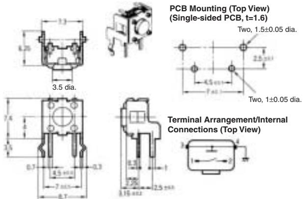
**Vertical, Flat Plunger Type (Height: 3.85 mm)**
