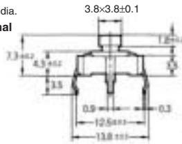
6 mm × 6 mm Radial Types (Taping Specifications): Sold in Units of 1,000 Switches
