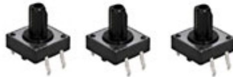
Figure 3.2. S.P.S.T. momentary, normally open. 0.48" square x 0.18" body. Plunger stands 0.3" above body. Four PC leads on 0.2" x 0.5" centers. CAT# MPB-127, http://www.allelectronics.com .
