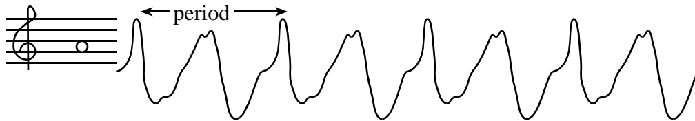
Figure 6.3. A waveform shape that generates a trumpet sound.
