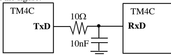
**Estimate** the fastest baud rate that can be implemented reliably. Show both your work and your estimate of maximum baud rate in bits/sec. time constant is  $10\Omega * 10nF = 100ns$ , we pick a baud rate about 10 times slower than time constant. So the baud rate should be 1 Mbps or slower.
