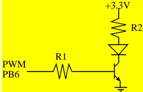
If you were to try to do this with a DAC, you would need to run the TIP120 in linear region. It would be almost impossible to match the nonlinearity of LED brightness with the nonlinearity of the TIP120 circuit. PWM with saturated TIP120 gives precise and linear control over brightness.
