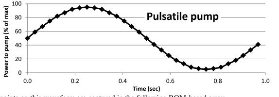
The points on this waveform are captured in the following ROM-based array. uint8\_t const Wave[32] = {50,59,67,75,82,87,92,94,95,94,92,87,82, 75,67,59,50,41,33,25,18,13,8,6,5,6,8,13,18,25,33,41};
