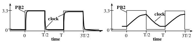
Slower than 250kHz, f=125 kHz, the signal looks ok. Each pulse is  $4\tau$ , 1-e<sup>-4</sup> = 0.98. This means 0.98\*3.3V = 3.24V, which means the clock will oscillate between 0.03V and 3.27V
