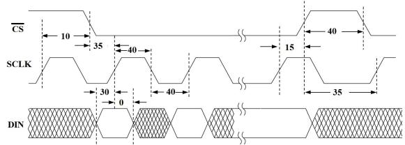
(2) Part a) What is the setup time for the MAX549A? Give the number in ns.
