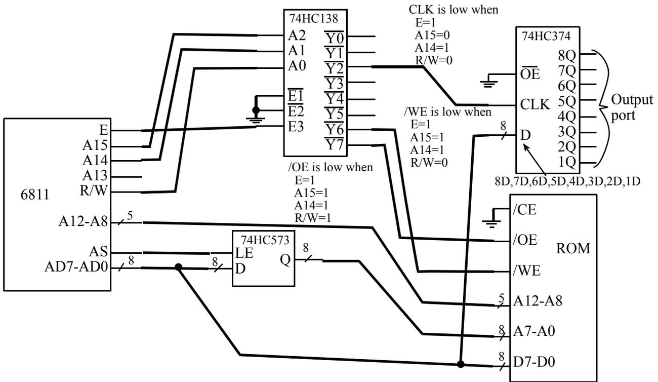
**Part d)** The rising edge of CLK stores into the 374 with a setup of 30 and a hold of 5ns
