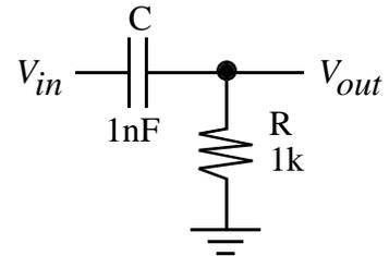
**(5) Part b)** Draw a rough plot of the gain ( $|V_{out}/V_{in}|$ ) versus frequency for the circuit. Include three points,  $f=0$ ,  $f_c$  (the point where is gain is  $\text{sqrt}(2)/2=0.707$ ), and at very large  $f$ . What is the value of  $f_c$ ?
