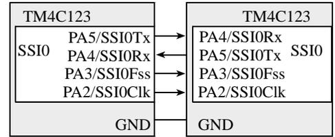
**Part a)** Assume the master (one on the left) has **SPH=1**, **SPO =0**, and **DSS=15** in the **SSI0\_CR0\_R** register. What are the correct configurations for **SPH**, **SPO**, and **DSS** in the slave (one on the right)?
