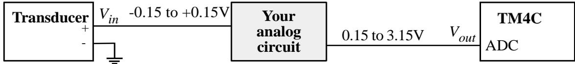
Your job is to design the analog circuit that implements  $V_{out} = 10 \cdot V_{in} + 1.65V$ . The input voltage varies from -0.15 to +0.15V, so the output voltage will vary from 0.15 to 3.15V. The output,  $V_{out}$ , is connected to the microcontroller ADC. R1 and R2 are already chosen such that the analog reference is 1.65V. You may use any chips shown in the book or presented in class. Show your work and label all chip numbers and resistor values. You do not have to show pin numbers.
