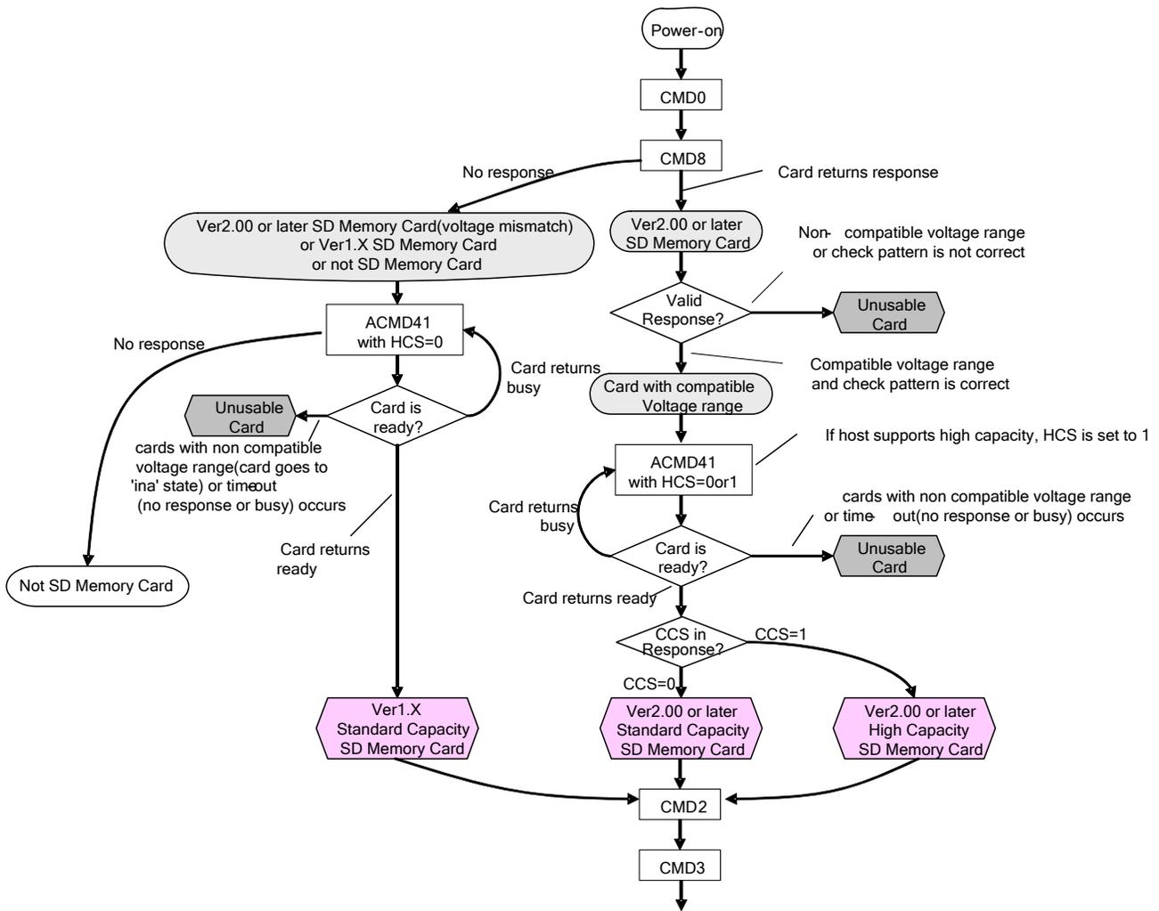
**Figure 4-2: Card Initialization and Identification Flow (SD mode)**
