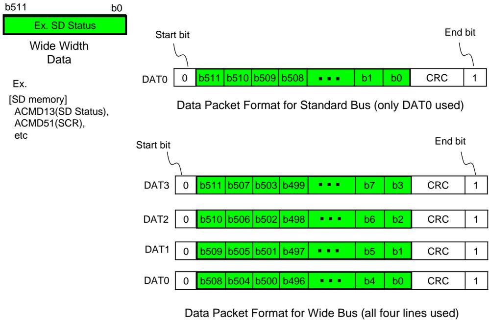
**Figure 3-8: Data Packet Format - Wide Width Data**
