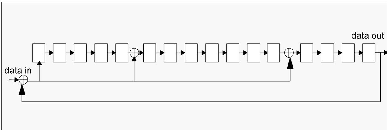
**Figure 4-7: CRC16 Generator/Checker**
