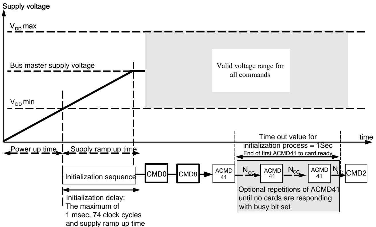
**Figure 6-1: Power-up Diagram**
