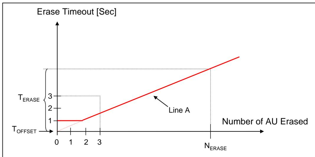
Figure 4-10: Example Erase Characteristics (Case 1  $T_{OFFSET}=0$ )
