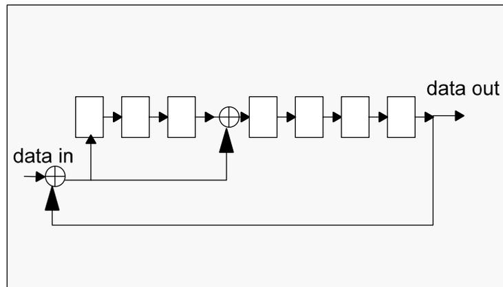
**Figure 4-6: CRC7 Generator/Checker**
