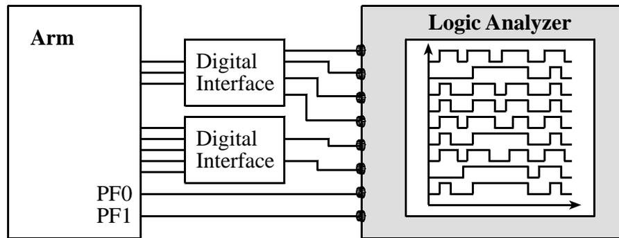
*A logic analyzer and example output.*
