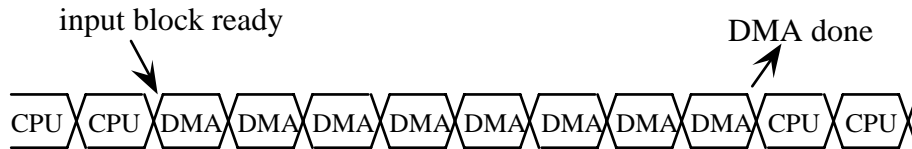
Figure 13.13. An input block is transferred all at once during burst mode DMA.
