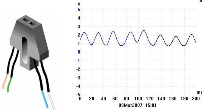
Tachometer data collected with a 15-slot disk powered at +9V. IR sensor interface on left
