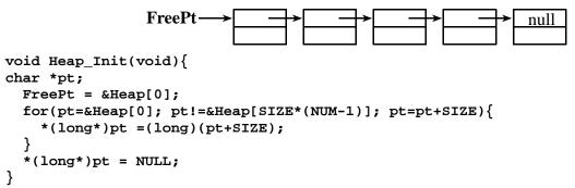
To allocate a block to manager just removes one block from the free list. The **Heap\_Allocate** function will fail and return a null pointer when the heap becomes empty. The **Heap\_Release** returns a block to the free list. This system does not check to verify a released block actually was previously allocated.
