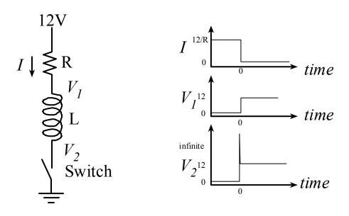
Start with the current. Initially the current is +12/R. Since the switch is ideal the current flips to zero at time  $0^+$ . Since the resistor is ideal, the voltage  $V_1$  simply goes from 0 to 12V. The voltage across the inductor goes to –infinity at time = 0 because the dI/dt is infinite. Therefore the voltage at  $V_2$  ideally becomes infinite at  $t=0^+$ , which is why we add the 1N914 snubber diode.
