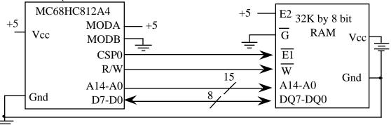
Part a) Except for the number of address lines and the specific timing values, you may assume your 32k RAM is identical to the 60L64 8k RAM shown in section 9.7.2. You may also assume  $t_{AVQV}$  equals  $t_{E1LQV}$ . Assuming you will be running with 3 cycle stretches, what is the maximum (slowest) access time  $t_{AVQV}$  that can be used?
