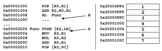
(6) Part a) Give the state of the stack (SP and contents) after executing of the PUSH instruction, as shown by arrow A: pop (R0,R1) causes R0=2, R1=3, SP=0x20001000
