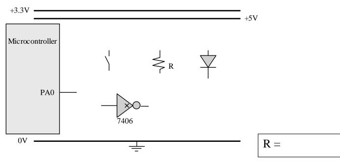
(5) Question 7. You are to interface an external Switch on Port A pin 0 that operates using negative logic by using the needed elements in the following figure. Given the TM4C microcontroller limits the current flow into it to  $2 \mu A$  calculate the voltage at Port A pin 0 when the switch is open. Choose a value for R and specify its value.
