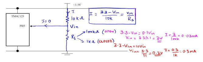
Assume no current can flow into or out of the port pin. The on-resistance of the switch is **not** 0 ohms and the off-resistance is **not**  $\infty$  ohms. Rather, the resistance of this switch is 1  $k\Omega$  when closed and 100  $k\Omega$  when open. Find the current through the switch and the voltage across the switch for the open and closed conditions. Complete the following table. Show the equation and then do the math to calculate the numbers.
