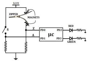
A switch S (interfaced on PD1, creating signal A), serves as an Off/On switch to disable or enable the system. The microcontroller reads an open switch S as disable and a closed switch S as enable of the BZBD system. There are two LEDs interfaced (red on PD2 and green on PD3) that indicate whether the zipper is breached (Red ON, Green Off) or is secure (Red Off, Green On). When the system is disabled both LEDs must be Off.
