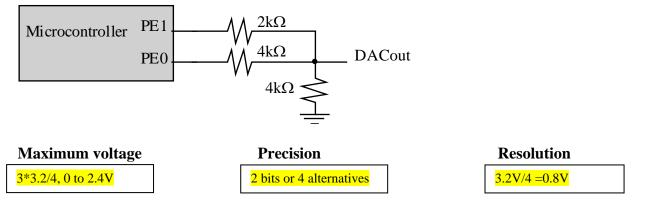
Solve for output  $01_2$ , 2k in parallel with 4k is (2\*4/(2+4))=1.333k. 3.2V-4000-1.333-ground, so DACout is 3.2V\*1.333/5.333=0.8Solve for output  $10_2$ , 4k in parallel with 4k is 2k. 3.2V-2000-2000-ground, so DACout is 3.2V\*2000/4000=1.6Max output is  $11_2$ , 0.8+1.6=2.4V
