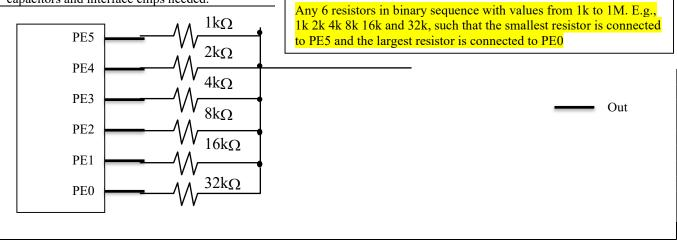
(10) Problem 3: Design a 6-bit DAC connected to Port E using PE5 to PE0. Show the circuit and label all resistors, capacitors and interface chips needed.
