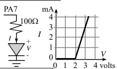
I = 3 \* (V - 2), where I is in mA, V is in volts.
