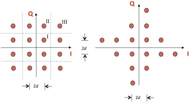
Energy in the pulse shape is 1. Symbol time  $T_{\text{sym}}$  is 1s. The constellation on the left includes the decision regions with boundaries shown by the in-phase (I) axis, quadrature (Q) axis and dashed lines.
