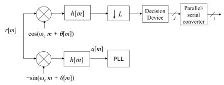
$\theta[m]$  is the carrier phase offset, and h[m] represents a lowpass finite impulse response (FIR) filter.
