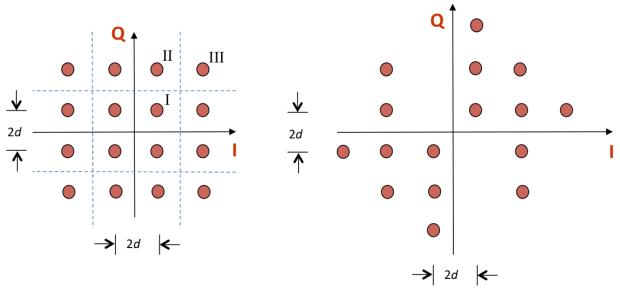
Energy in the pulse shape is 1. Symbol time  $T_{\text{sym}}$  is 1s. The constellation on the left includes the decision regions with boundaries shown by the in-phase (I) axis, quadrature (Q) axis and dashed lines.
