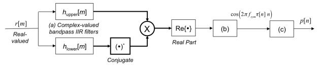
Upper filter  $h_{upper}[m]$  locks onto (passes) continuous-time frequency  $f_c + \frac{1}{2} f_{sym}$  and the lower filter  $h_{lower}[m]$  locks onto (passes)  $f_c - \frac{1}{2} f_{sym}$ . The thicker/bold lines indicate complex-valued signals.
