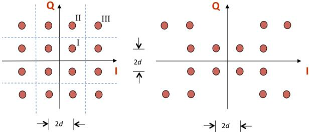
Energy in the pulse shape is 1. Symbol time  $T_{\text{sym}}$  is 1s. The constellation on the left includes the decision regions with boundaries shown by the in-phase (I) axis, quadrature (Q) axis and dashed lines.
