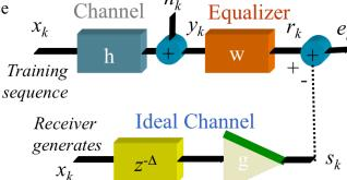
(b) Here is the update equation for an adaptive least mean squares FIR filter with N coefficients w:
