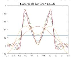
The approximated function is shown using 21 Fourier synthesis terms (N=10) on the left and 201 Fourier synthesis terms (N=100) on the right:
