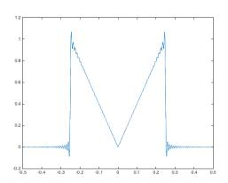
On the right, Gibbs phenomena occur at the amplitude discontinuities at  $-0.25T_0$  and  $0.25T_0$ . At these points, there is an 8.9% error at the value of 1 and 8.9% error in the value of 0.
