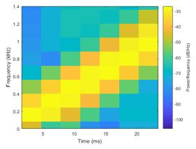
In this case, it is difficult to get a well-defined spectrogram because we only have 200 samples to work with and the chirp is increasing its frequency quickly over the 200 samples.
