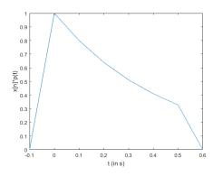
**Epilogue:** Here we see that different interpolation functions give very different reconstructed signals. In lecture, we have also discussed sinc interpolation, which can perfectly reconstruct a bandlimited signal.
