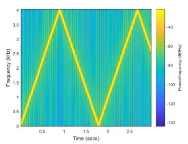
To explain this plot, first calculate the maximum frequency without aliasing effects as we did in part (b) above. In this part,  $T_{\text{max}} = 24000 \, T_{\text{s}} = 24000 \, f_{\text{s}} = 3 \, \text{s}$  and the maximum instantaneous frequency is  $f_{\text{max}} = (44.8 \times 10^2) \, T_{\text{max}} = 13.44 \, \text{kHz}$  which means  $f_{\text{max}} / f_{\text{s}} = 1.68$ . The sampling theorem is not followed for continuous-time frequencies at or above 4 kHz.
