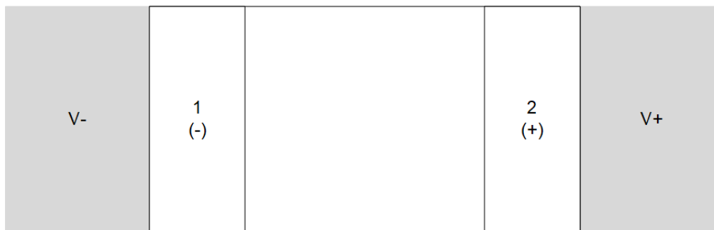
Figure 8-14. Recommended Layout: DEC Package
