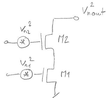
$$V_{nout}^2 = V_{n2}^2 \cdot (g_m r_{o2})^2 + V_n^2 (g_{m2} r_{o2} g_{m1} r_{o1})^2$$
