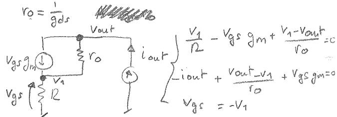
$$\text{Subs. } \left\{ \begin{array}{l} -\frac{V_{gs}}{R} - V_{gs} g_m - \frac{V_{gs} + V_{out}}{r_o} = 0 \\ -i_{out} + \frac{V_{out} + V_{gs}}{r_o} + V_{gs} g_m = 0 \end{array} \right.$$
