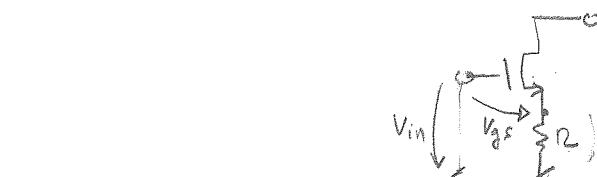
$$\frac{V_{gs}(\frac{1}{r_o} + g_m)}{V_{gs}(\frac{1}{R} + g_m + \frac{1}{r_o})} = \frac{i_{out} - \frac{V_{out}}{r_o}}{-\frac{V_{out}}{r_o}}$$
