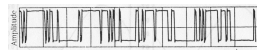
B Dither of one-third LSB rms amplitude is added to the sine wave before quantization, resulting in a PWM waveform.
