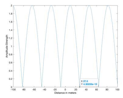
In the Matlab plot, we've used the Data Cursor tool (under the Tools menu in the Matlab plot window) to show the value of x (distance) at 27.5 m where the value of y (Amplitude Strength) is zero. Please note that  $4.3 \times 10^{-13}$  is essentially zero. This number is not equal to zero due to the numerical accuracy in double-precision floating-point calculations.
