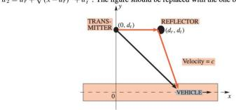
The received signals the sum of the two copies, and since they travel different distances they have different time delays. If the transmitted signal is s(t), then the received signal is
