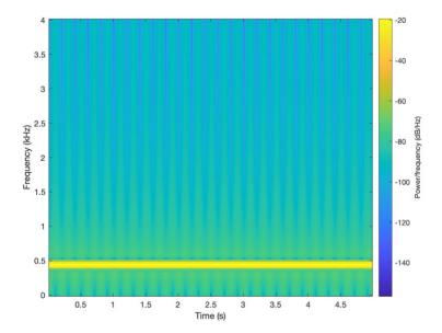
x(t) only contains frequencies  $\pm 440$  Hz, and the spectrogram shows this. The spectrogram, by default, only shows non-negative frequencies, and the plot over negative frequencies will be a mirror image of the positive frequencies.
