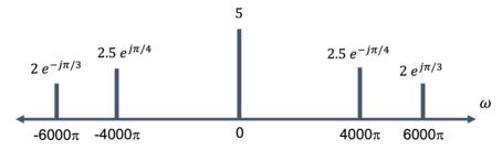
**Solution:** The above spectrum indicates that the signal has frequency components of  $-6000\pi$  rad/s,  $-4000\pi$  rad/s, 0 rad/s,  $4000\pi$  rad/s and  $6000\pi$  rad/s. The strongest frequency component is at 0 rad/s because its magnitude (5) is the largest. The second strongest frequency components are at  $-4000\pi$  rad/s and  $4000\pi$  rad/s. The weakest frequency components are at  $-6000\pi$  rad/s and  $6000\pi$  rad/s.
