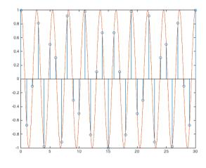
**Epilogue:** For a sinusoidal signal with discrete-time frequency  $\widehat{\omega}_0 = 2\pi \frac{f_0}{f_s} = 2\pi \frac{N}{L}$  where the common factors in  $f_0$  and  $f_s$  have been removed so that N and L are relatively prime, the discrete-time signal has a fundamental period of L samples. The fundamental period of L samples contains N periods of a continuous-time sinusoid with frequency  $f_0$ . Please see <u>Handout D on Discrete-Time Periodicity</u>.
